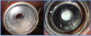
ON LEFT: Volute shows signs of severe wear. ON RIGHT: Cycloseal<sup>®</sup> backplate still has primer on it.
