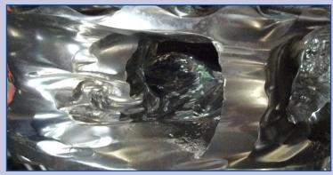
Impeller scoured by the sand mixture
